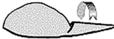
sandbag, open end folded over - side view
