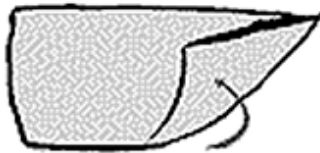
sandbag, 1/3 full, open end folded over - top view
